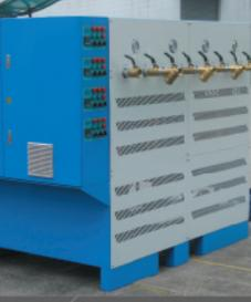
橡胶四辊压延机温控TCU
